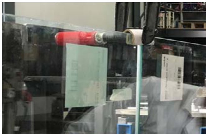
Figure 6: Connect adjacent panes using F-clamps
