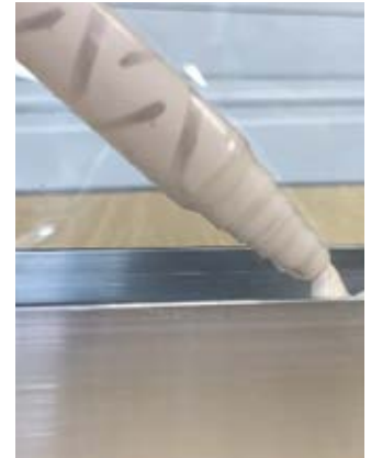
Figure 11: Injecting the mixed part A and part B in the U-profile
