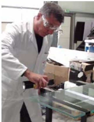
Figure 3: Spray release agent on glass
